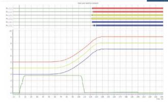
Fig. 1: Timing measurement during a close operation shows failure in blue phase.
