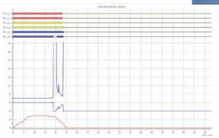
Fig. 2: Dynamic resistance measurement shows failure in blue phase.
